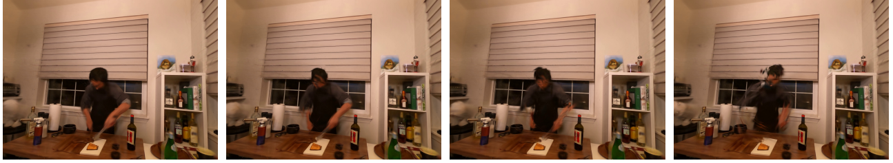
Figure 10. Without Gaussian waypoints, long forward integration causes rollouts to slowly drift and distort the scene
